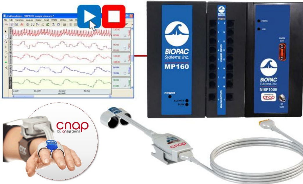
NIBP100E module (right) shown with MP160 data acquisition system
